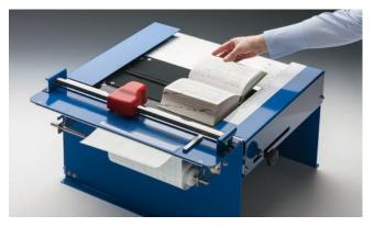
Please ensure that there is an overlap here, too, of 2 cm for the book cover. The distance between the edge and the head of the cutter should be about 2 cm. Open the book roughly at the middle and check the printed scale to see how much of the filmolux® film you will need to pull off the roll.
