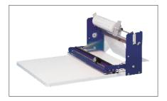
Fix a filmolux® film roll that is approx. 3-4 cm wider than the height of the book into the BLS-Classic. Peel the backing paper off the film.
