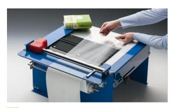
6. Pull the film off the roll to the measured coloured spot.
