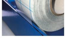
with the tape end to the back. Peel back approx. 15 cm of the release liner and feed the tape into the separator.
