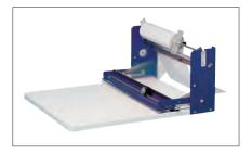
1. Fix a filmolux® film roll that is approx. 3 - 4 cm wider than the height of the book into the BLS-Classic. Peel the backing paper off the film.
