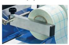
4. Secure the roll with the tape holder and tighten the screw. The tape can be cut off with a light diagonal, downward motion onto the cutting
