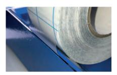
2. Place the tape roll in the seating tray with the tape end to the back. Peel back approx. 15 cm of the release liner and feed the tape into the separator.
