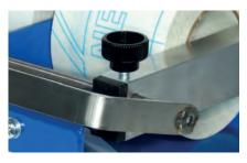
1. Loosen the knurled screw and slide the tape holder outwards.
